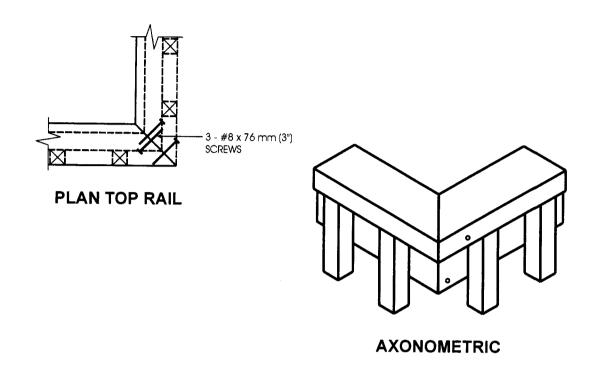
ONE FASTENER IN HORIZONTALLY ORIENTATED PORTION OF TOP RAIL AND TWO IN VERTICALLY ORIENTATED PORTION.
