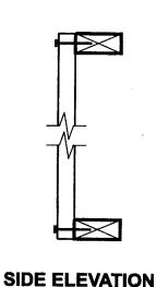
**Detail EC-3**Exterior Connection: Infill Picket Screwed to Rail
