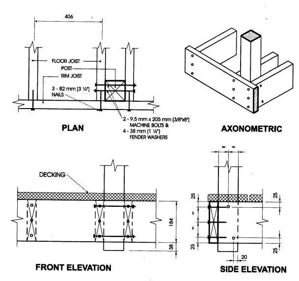
**Detail EB-5**Exterior Connection: Post Bolted to 2 Floor Joists
